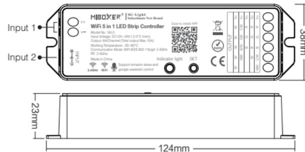
**SET Button:** Long press "SET" for 3 seconds; When red indicating light blink quickly, device reset and go into Smart Link mode.
