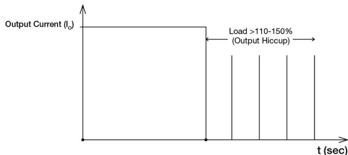
It is not recommended to prolong the duration of  $I_o$  when it is <110-150% but >100%, since it may cause damage to the PSU.
