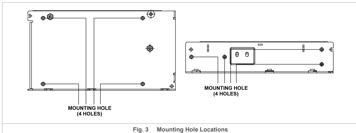
With reference to Fig. 3, the device should be mounted on a sturdy heat conducting surface with minimum of 4 mounting holes for base mounting or 3 mounting holes for side mounting. Use M3 screws only.
