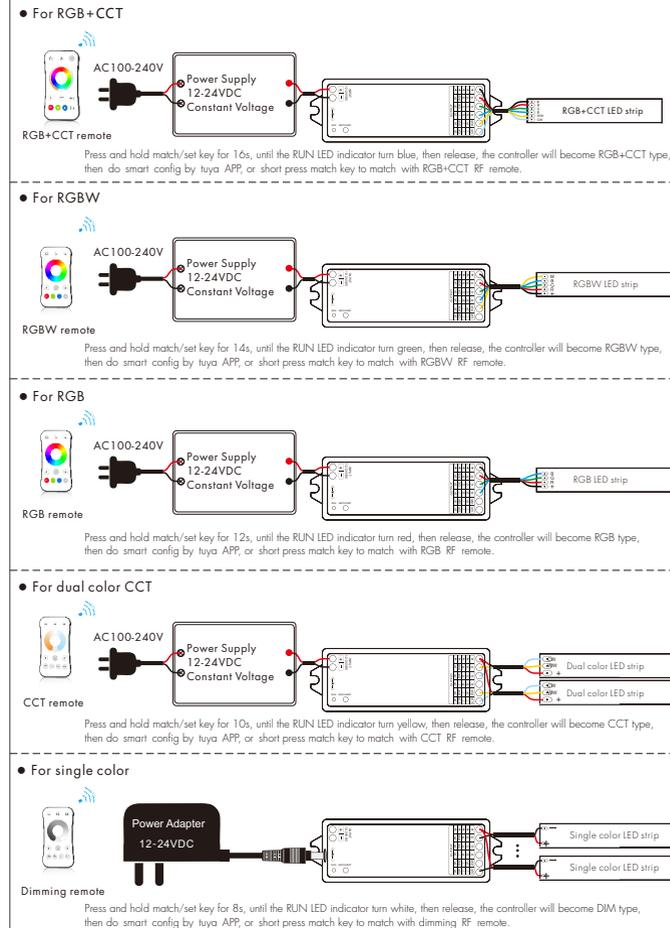
Note: User can connect constant voltage power supply or power adapter as power input.
