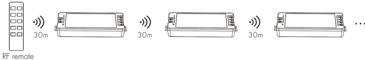
**Auto-transmitting:** One receiver can transmit the signals from the remote to another receiver within 30m, as long as there is a receiver within 30m, the remote control distance can be limitless.
